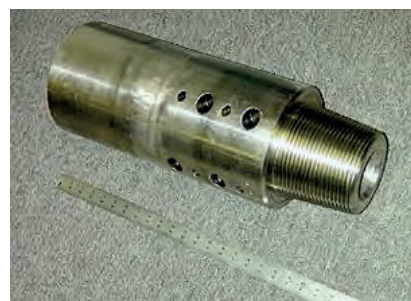
Fig 9. RM - Rotating Magnet – Prime Horizontal. Źródło: http://primehorizontal.com/hdd-guidance-services/hdd-coal-bed-methane/
